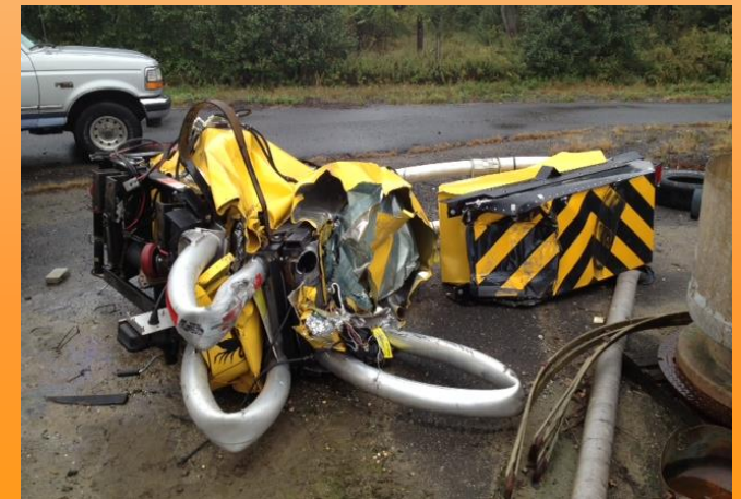
Driver hit the TMA truck at 55 MPH and was able to walk away unharmed.
